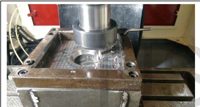
Fig. 8. Forming of parabolic cup on CNC machine.
